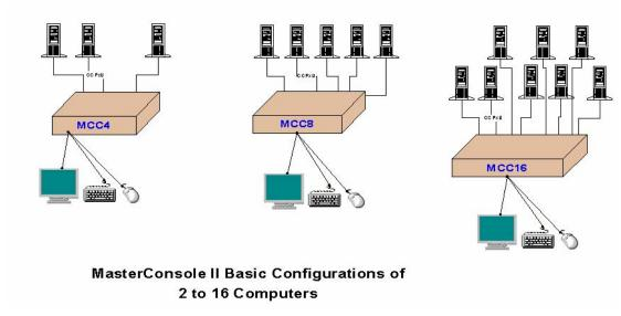
Figure 30 Basic One-Tier Configurations
